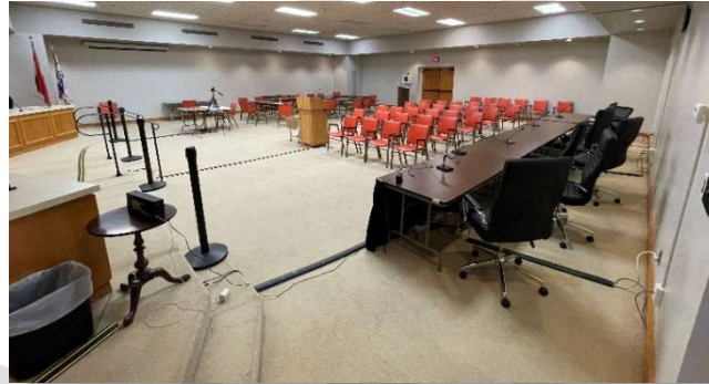
View of Council Chambers and wire raceways with wire and cables running on surface of floor being protected by tapered rubber covers.
