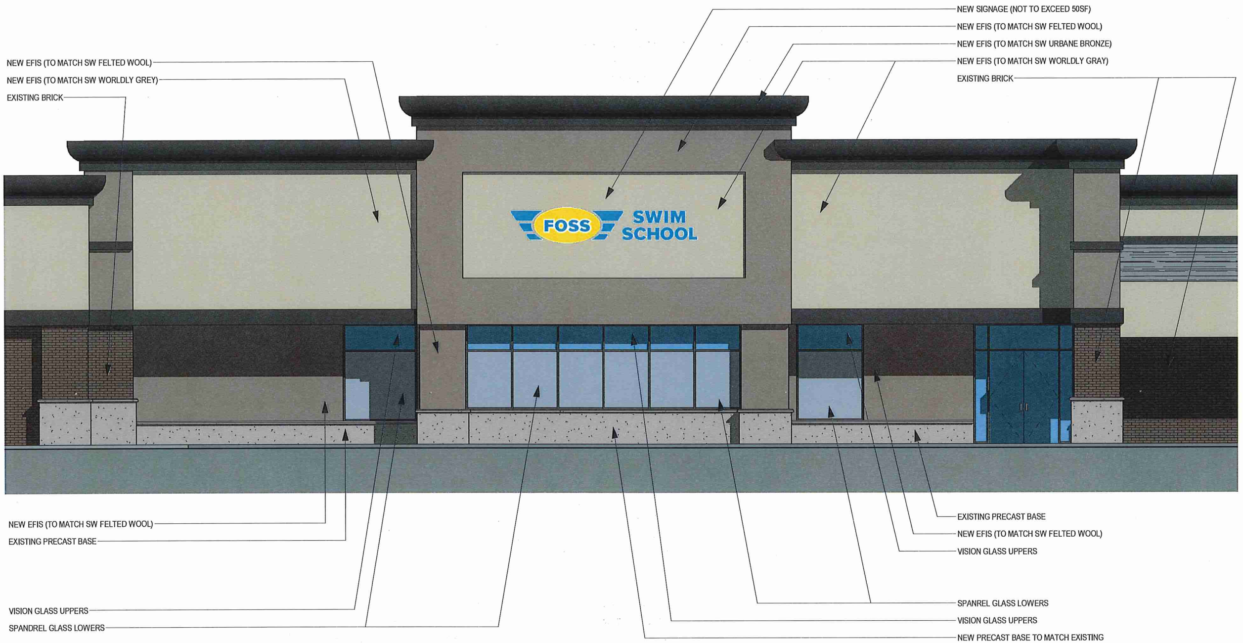
1 PRIMARY FACADE ELEVATION - NEW CONSTRUCTION A-2 1/8" = 1'-0"
