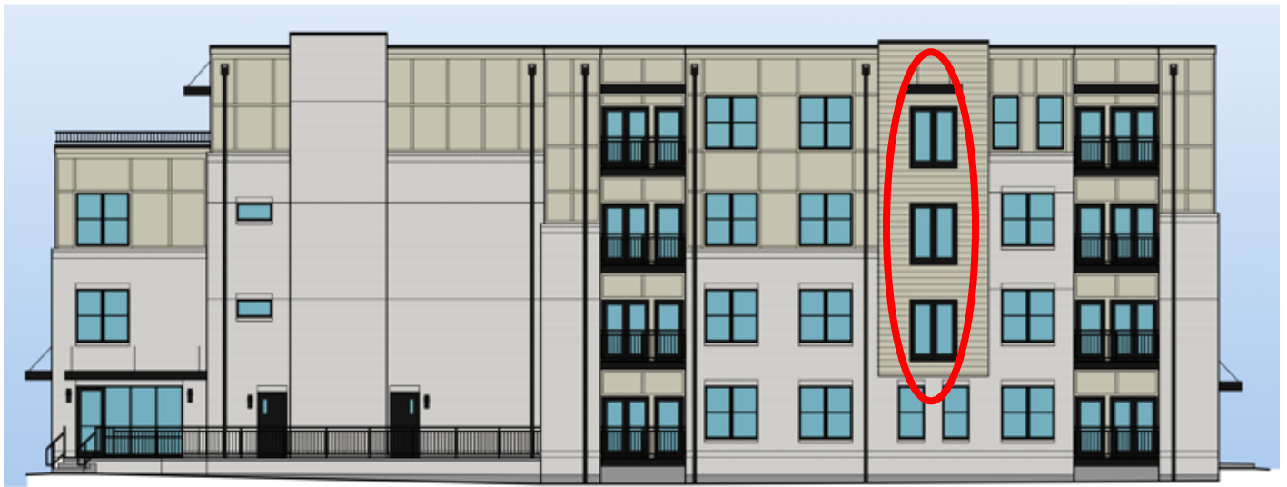
Figure 4: Rear/North Elevation proposed showing Juliette balconies removed.
