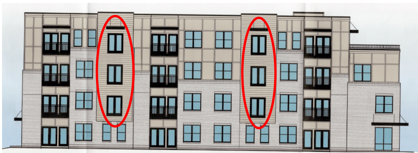
Figure 2: Front/South Elevation proposed showing Juliette balconies removed.
