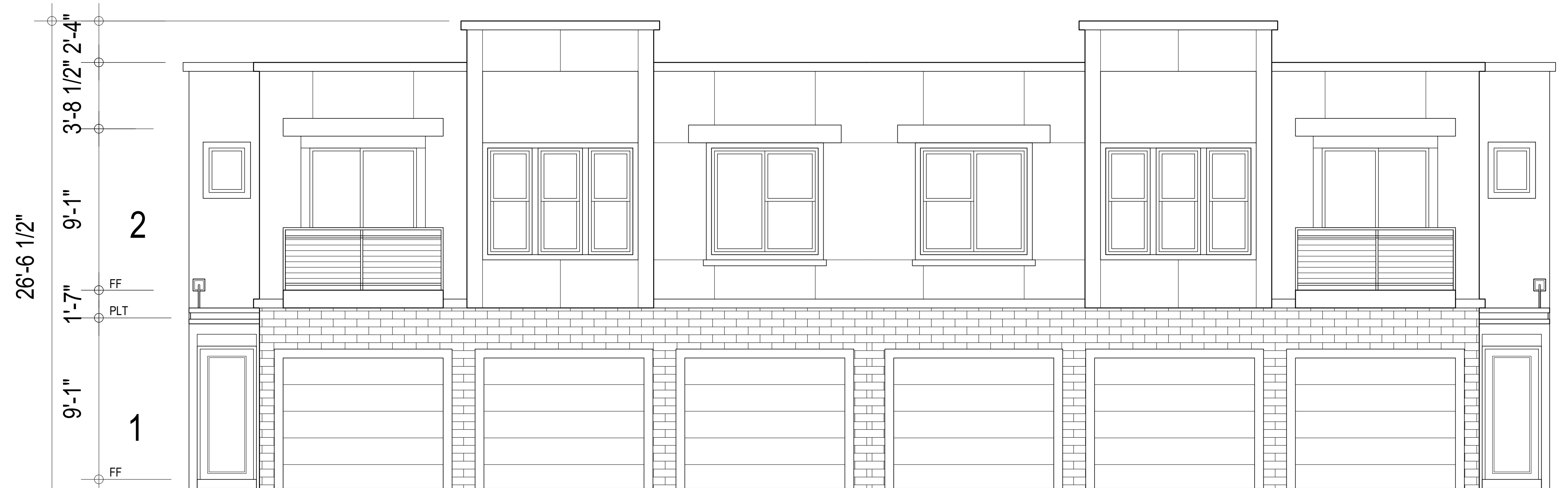
CARRIAGE HOUSE - FRONT ELEVATION SCALE: 1/4" = 1'-0" (24"x36" SHEET)
