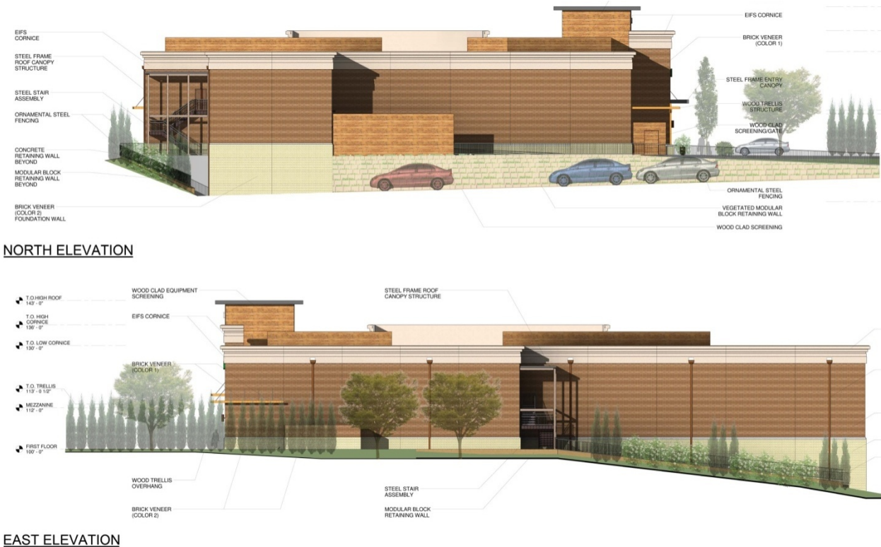
Figure 3: Note layers of surfaces and continuation of cornice around the building.
