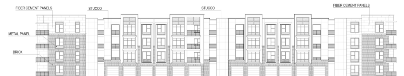
Figure 2: Elevation of the main residential building.
