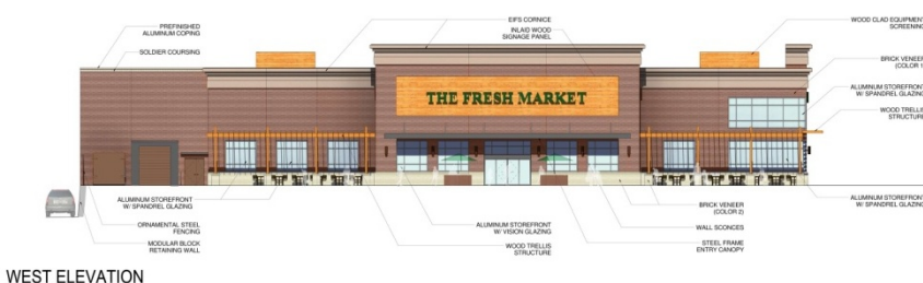
Figure 3. Note how the side façade treatment (right side of image) and the roof-top mechanical screen appear as appendages to the main structure rather than integrated into the structure.
