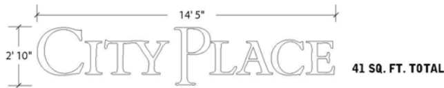
D WEST & SOUTH ELEVATION DETAIL: CITY PLACE CAMPUS IDENTIFICATION 1/4" = 1'-0"
