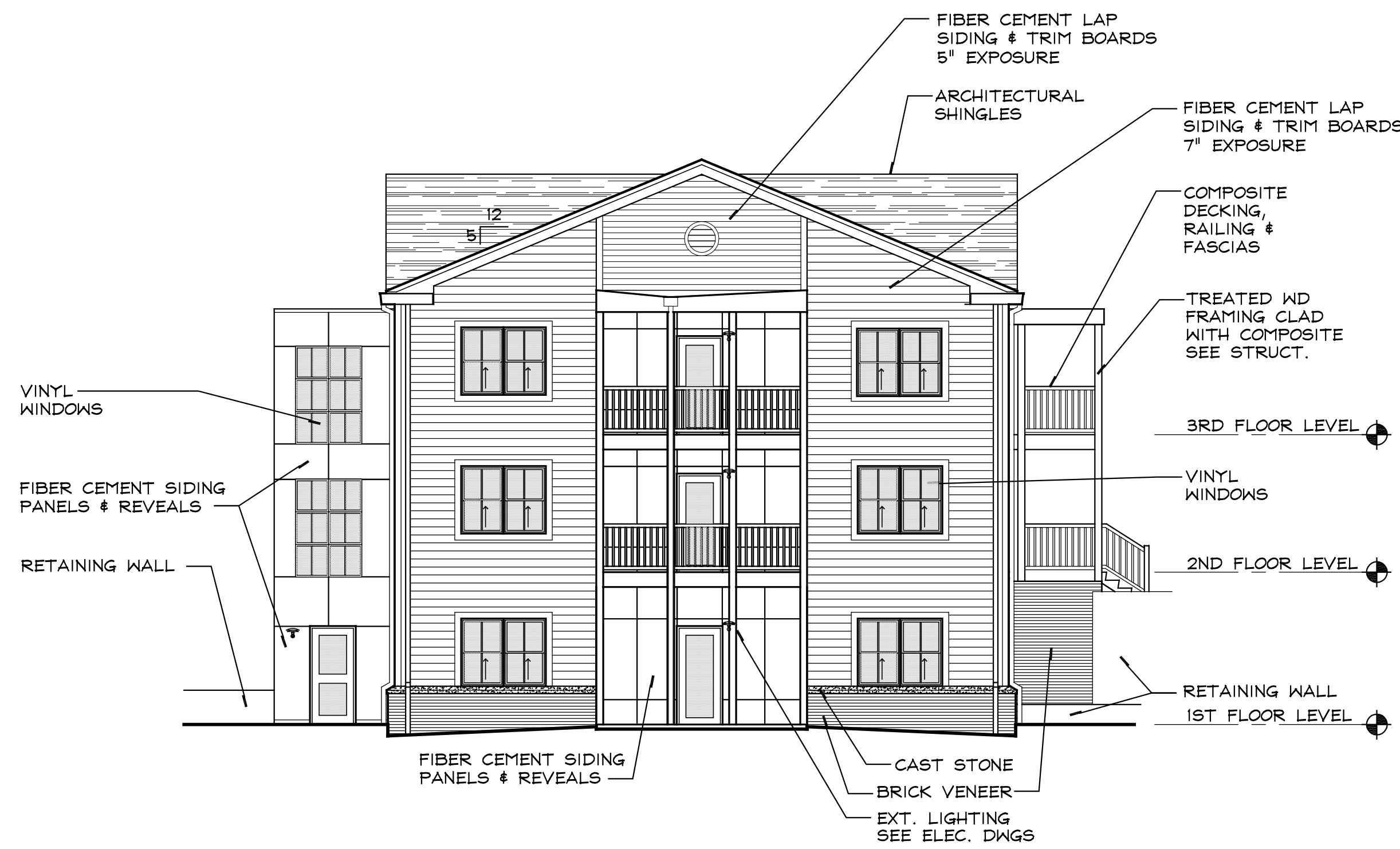
2 BUILDING 4 - NORTH ELEVATION A2.1 SCALE: 1/8" = 1'-0"
