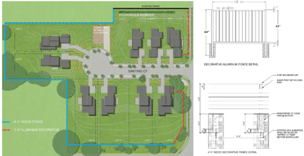
Figure 8: Original Fence Materials and Locations.
