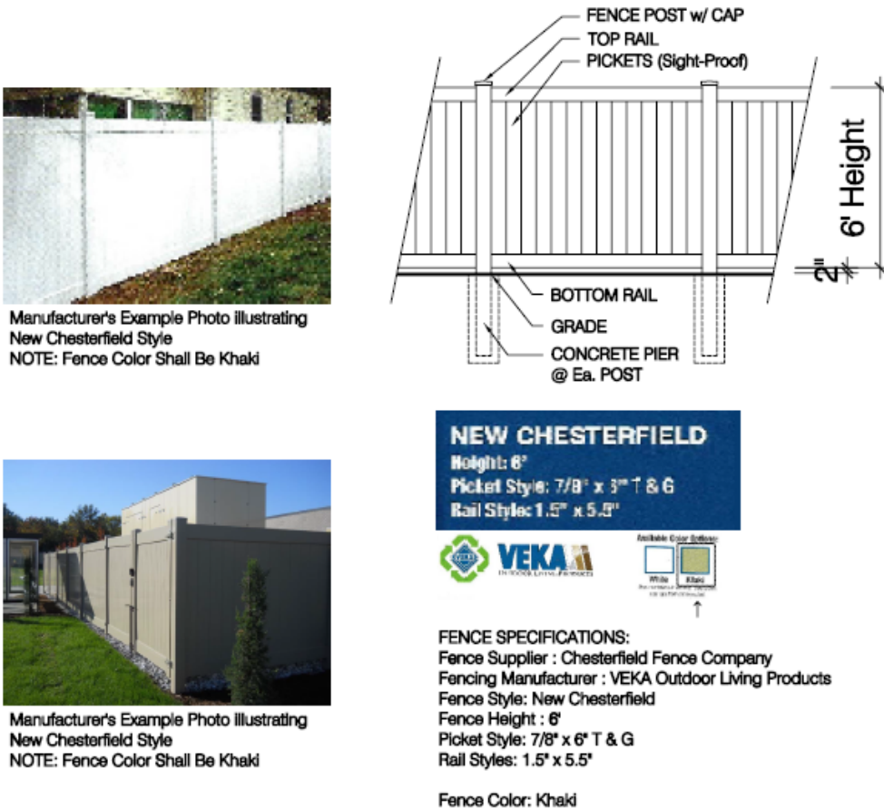
Figure 5: Fence Detail per Plans.
