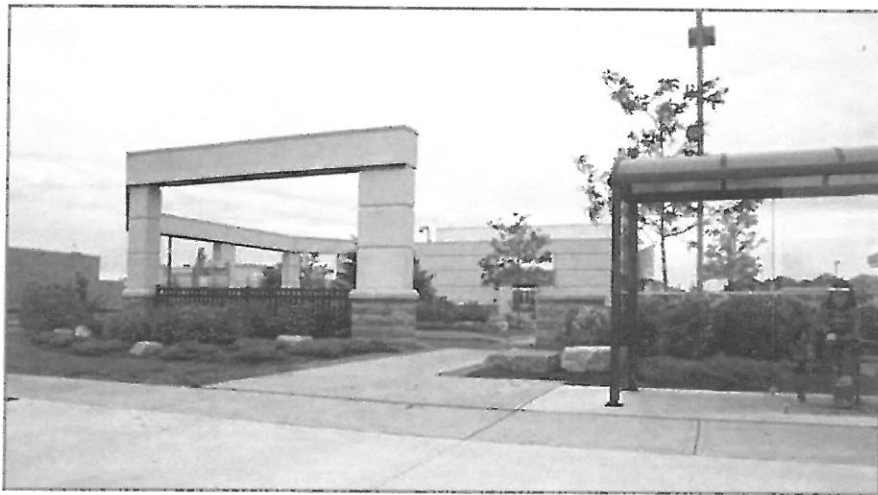
Figure 4.7g: This gas bar and drive-through facility at Bur Oak Avenue & McCowan Road utilizes an architectural screen to buffer the stacking lane from the street while maintaining a built form edge along the street.
