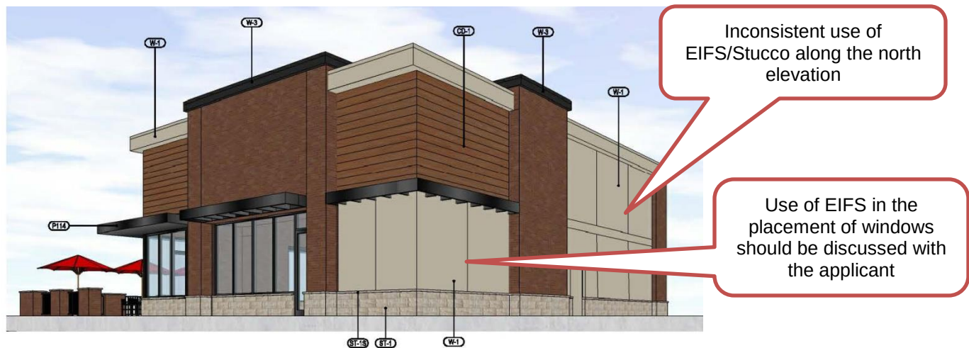
Figure 10: Northeast Corner Elevation
