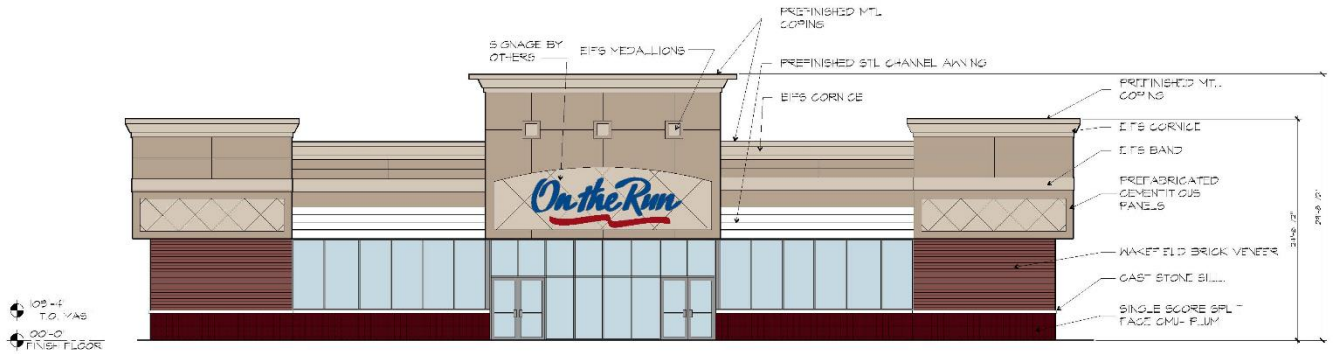
Figure 2: South Elevation of the Convenience Store
