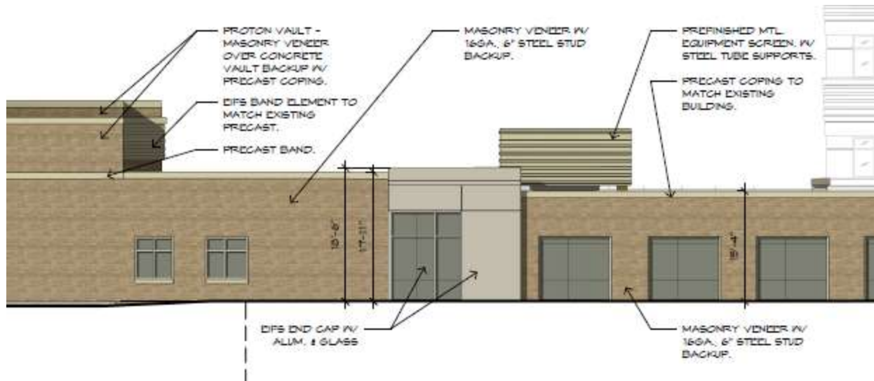
Figure 10: Close-up of the East Elevation of the mechanical screening.
