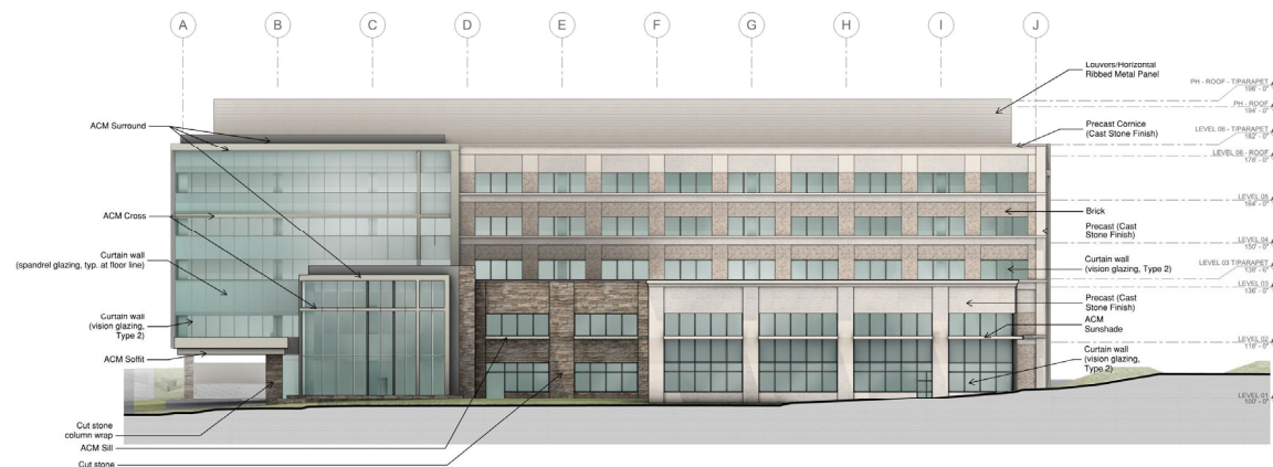
2 OVERALL BUILDING ELEVATION - EAST 1/8" = 1'-0"
