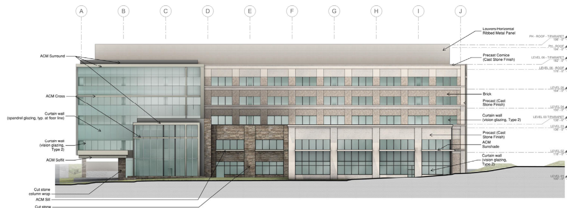
2 OVERALL BUILDING ELEVATION - EAST 1/8" = 1'-0"
