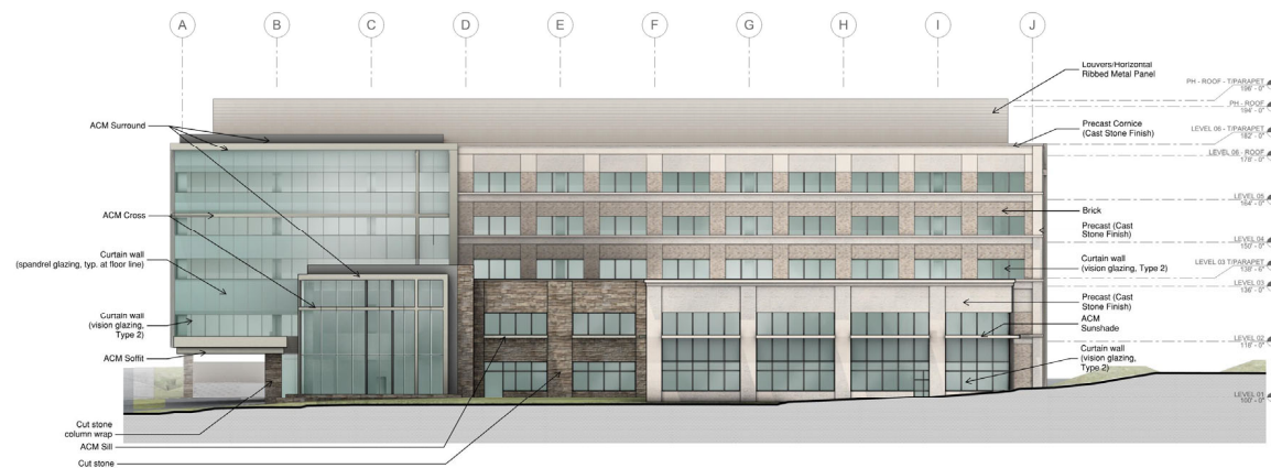
2 OVERALL BUILDING ELEVATION - EAST 1/8" = 1'-0"
