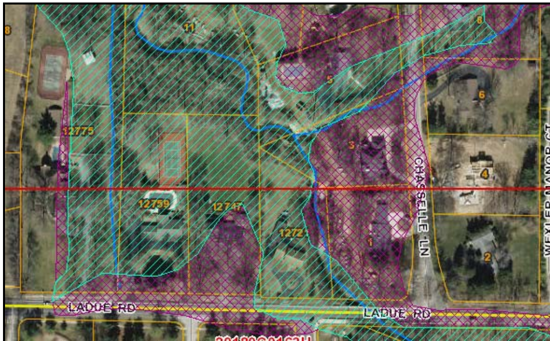
Figure 3: According to the existing floodplain maps, the creeks themselves (dark blue lines) are not in the flood plain (light blue hatching). Data source: St. Louis County website.
