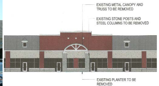
Figure 2: Close-up of existing elevation
