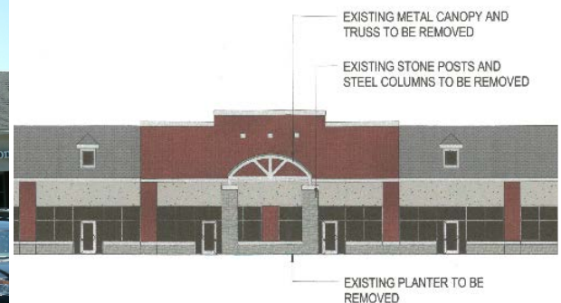
Figure 2: Close-up of existing elevation
