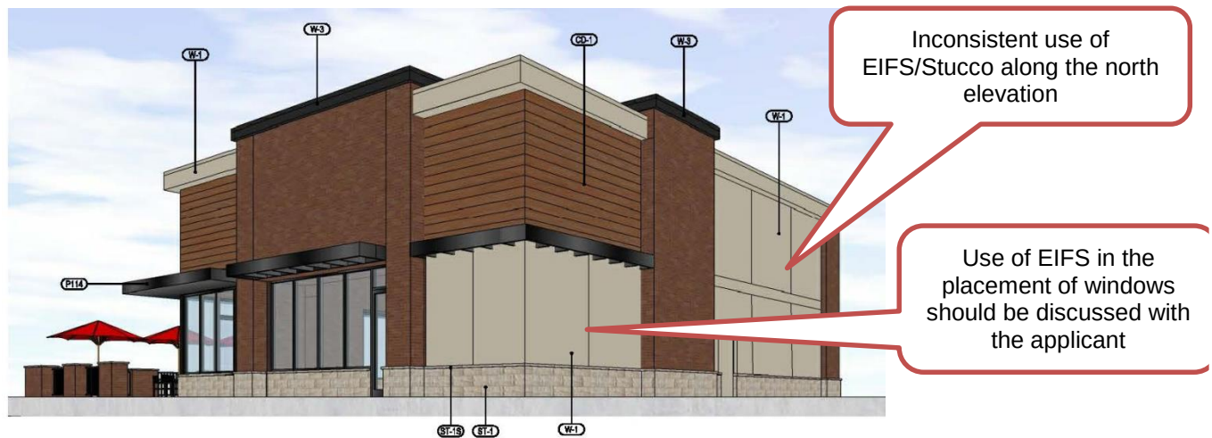
Figure 10: Northeast Corner Elevation
