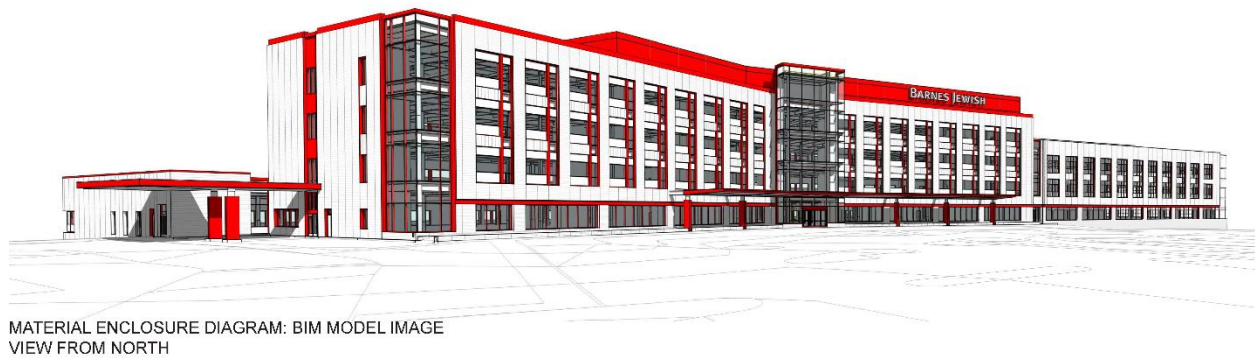
Figure 4: Applicants view indicating the use of the metal (shown in red) that is incorporated in the building and rooftop screen to create architectural consistency.
