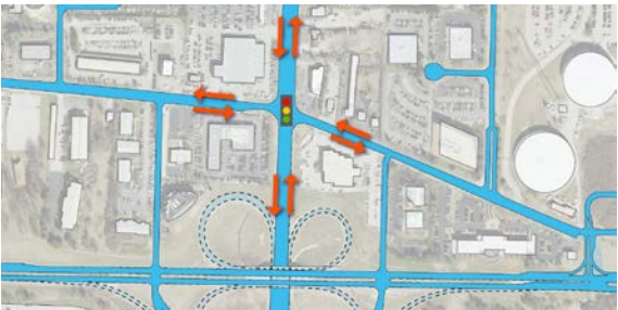
An at-grade signalized intersection.
