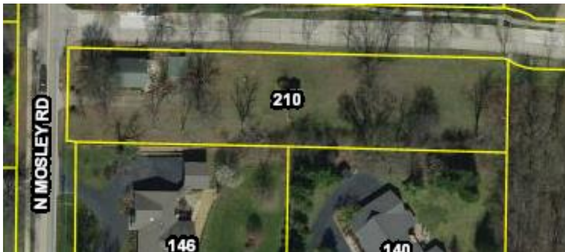
Figure 7: 210 N. Mason Road the original development established the side yard setback along the south property line. The existing home was then torn down and the new home was reoriented to the north.
