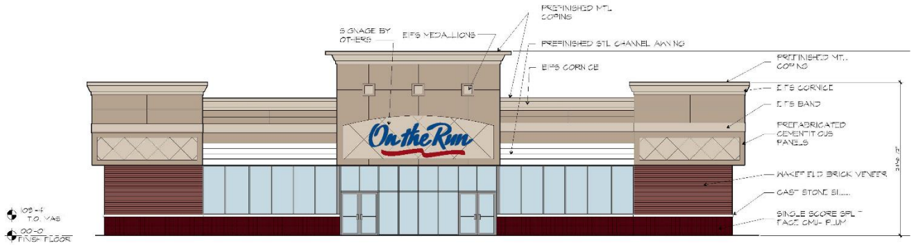
Figure 2: South Elevation of the Convenience Store
