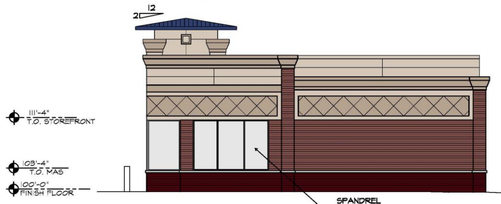
Figure 11: Close-up of the East Elevation showing the height of the storefront in comparison to the overall structure.
