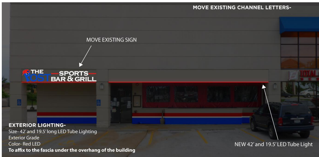
Figure 2: Detail of the Neon Style tube light along the exterior of the tenant space
