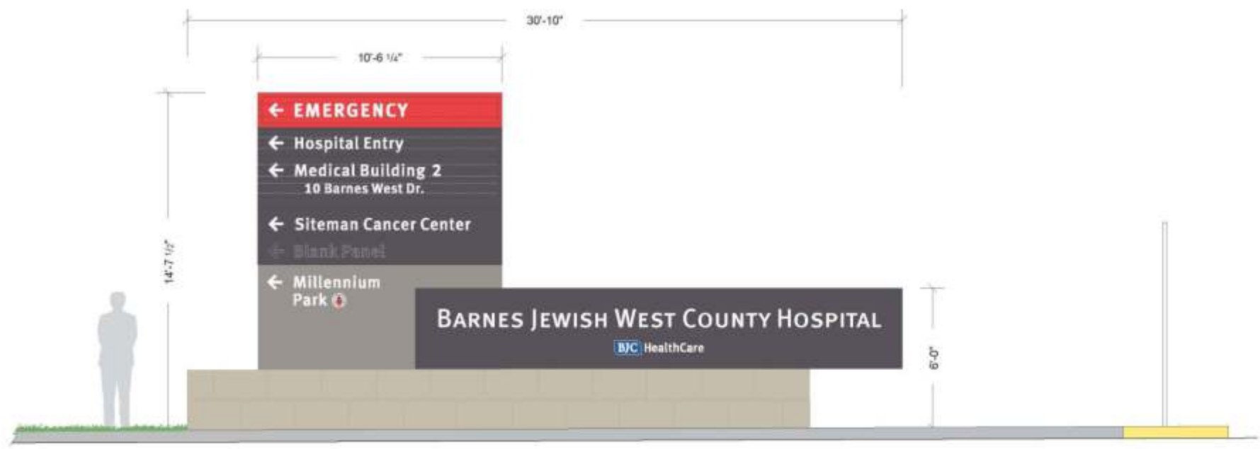
1 ELEVATION: BARNES WEST WAYFIND SIGN 8A SCALE: 1/4"=1'-0"
