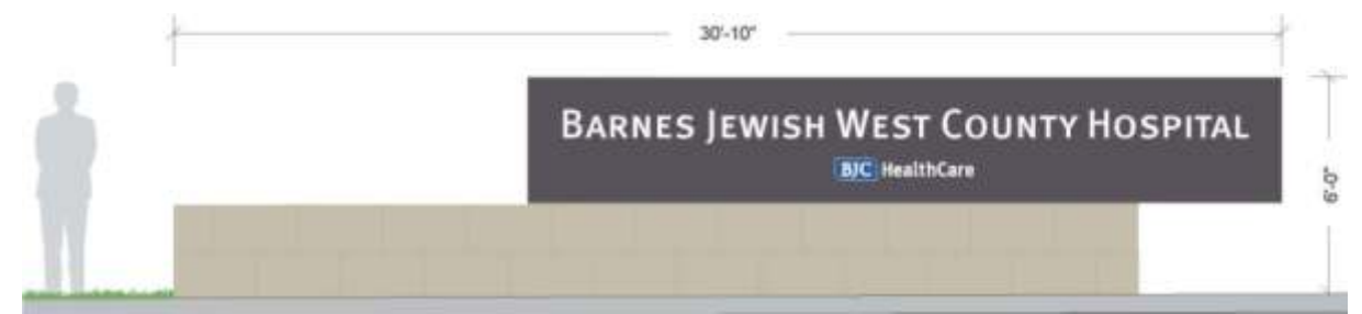
2 ELEVATION: BARNES WEST WAYFIND SIGN 8A SCALE: 1/4"=1'-0"
