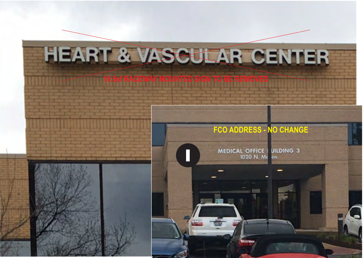
REMOVE & DISPOSE EXISTING CHANNEL LETTER SIGN 1'-0" X 19'-6" LEAVE NON-ILLUM. MOB 3 LETTERS AT ENTRY
