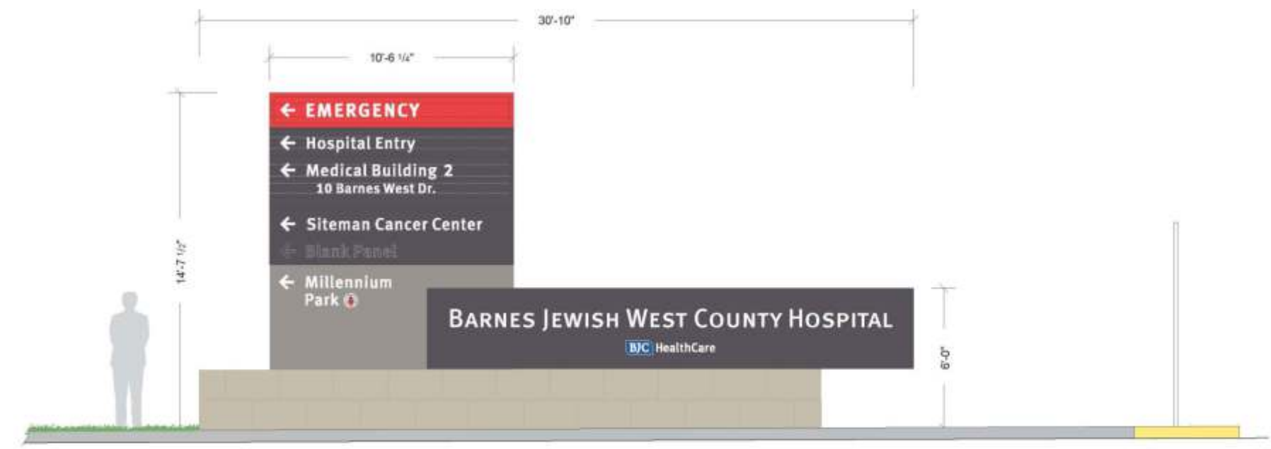
1 ELEVATION: BARNES WEST WAYFIND SIGN 8A SCALE: 1/4"=1'-0"
