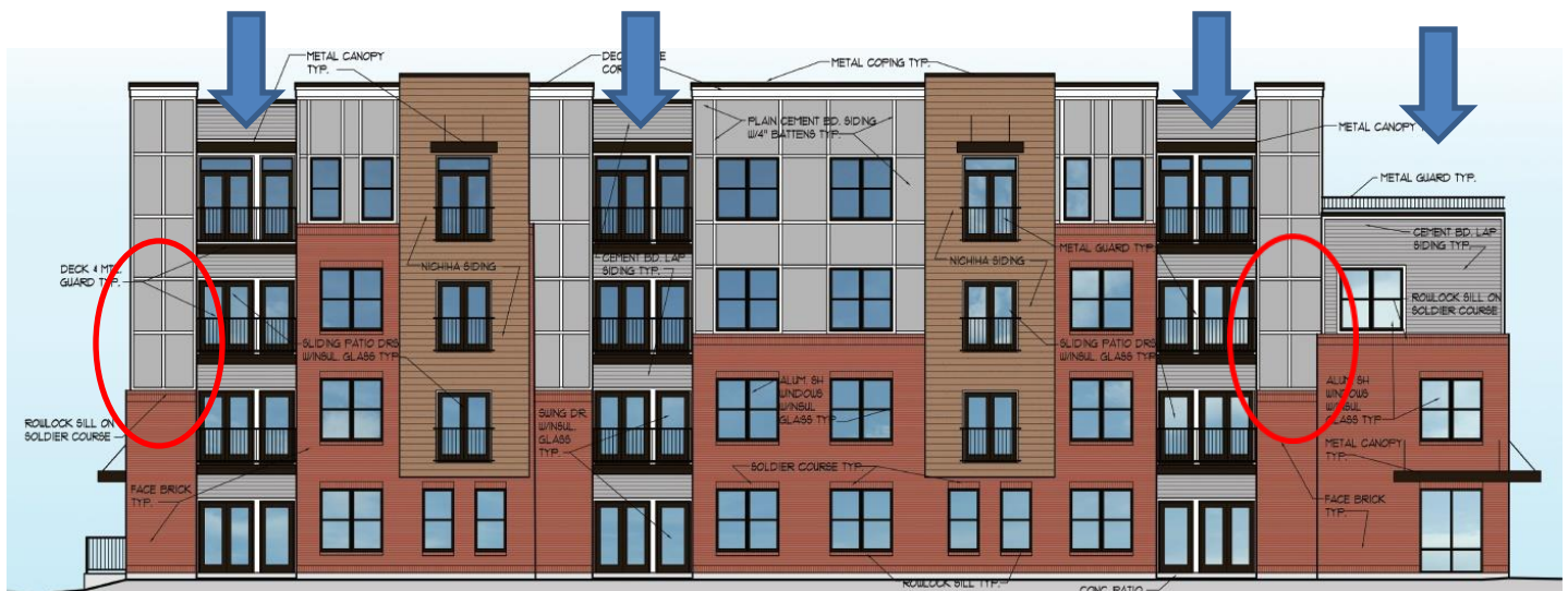
Figure 1: Previous South Front Elevation. Red circles indicate where the additional brick has been added. Blue arrows indicate the Lap siding that was removed and replaced with the plain cement building siding w/4" battens in a light grey with white trim,
