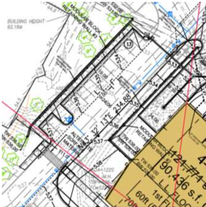
Figure 11: Close-up of the SDP showing the modular block walls on the west side of the building and on the adjacent property.
