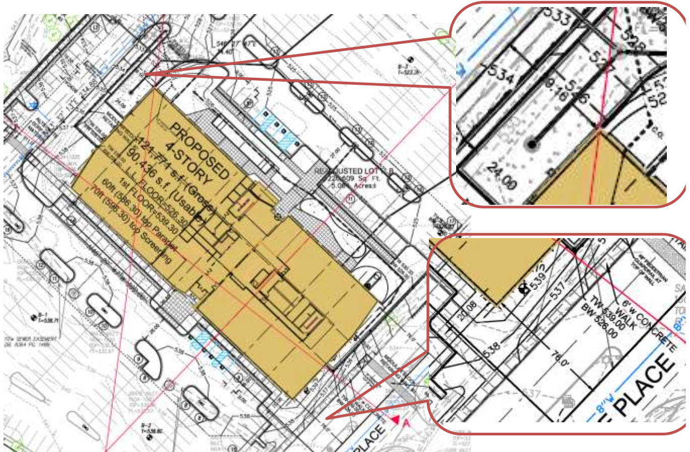
Figure 15: Close-up of the May 10 th site development plan of the proposed building, revised drawings received May 16 th , included a 5 foot strip to provide additional landscaping adjacent to the buildings.
