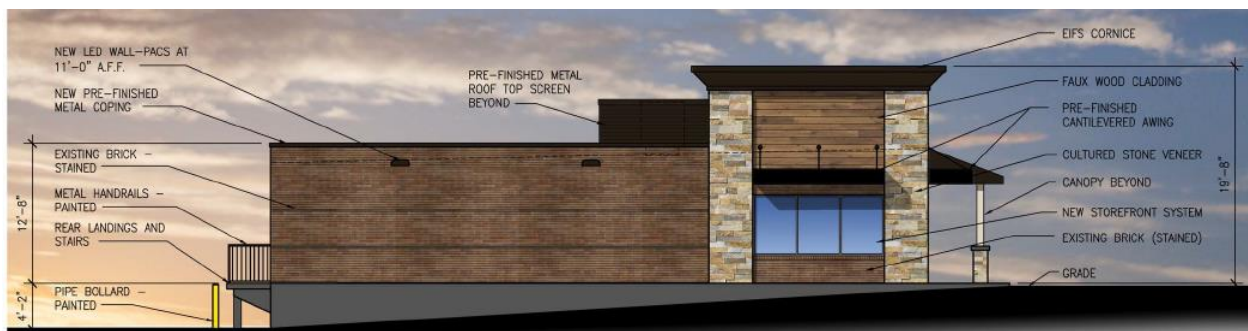
Figure 8: Close-up of the Side Elevation for the Retail Building
