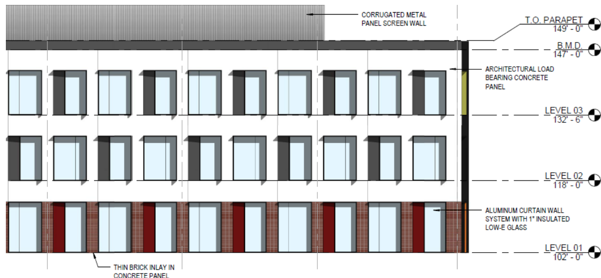
Figure 8: Close-up of the Elevations for the Office Building under construction.
