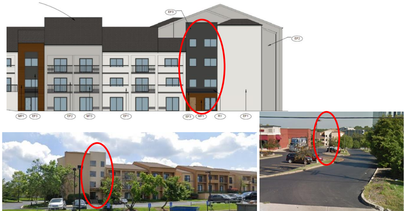
Figure 9: Close-up of the South Elevation at the east entrance where the cladding should be carried up to match the similar tower elements elsewhere, and Google images of the building from in front of 2 CityPlace and at the Aldi entrance on Olive Boulevard, with the area most visible.
