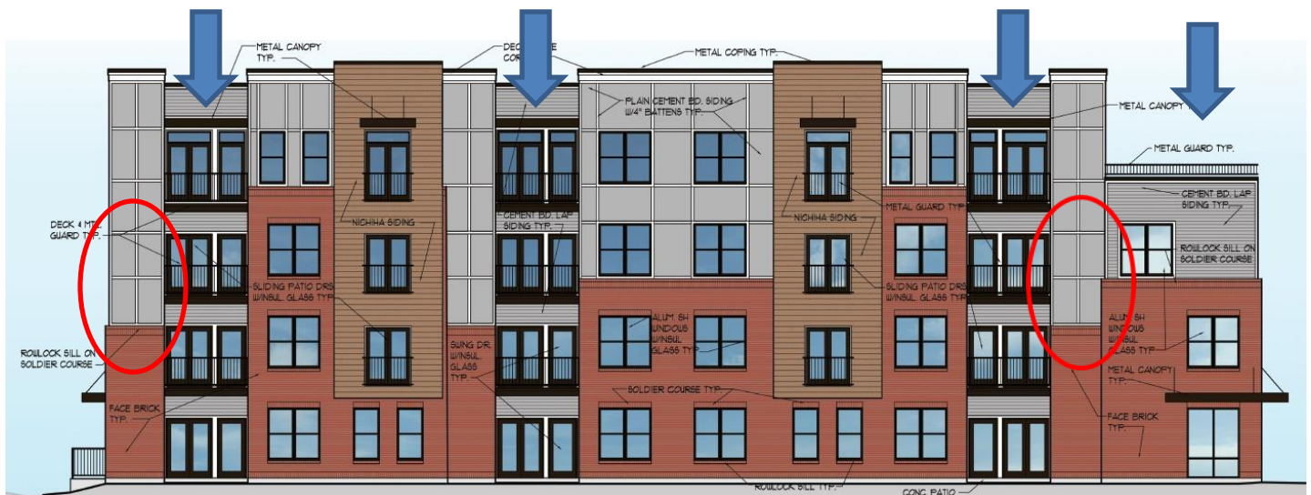
Figure 1: Previous South Front Elevation. Red circles indicate where the additional brick has been added. Blue arrows indicate the Lap siding that was removed and replaced with the plain cement building siding w/4" battens in a light grey with white trim,
