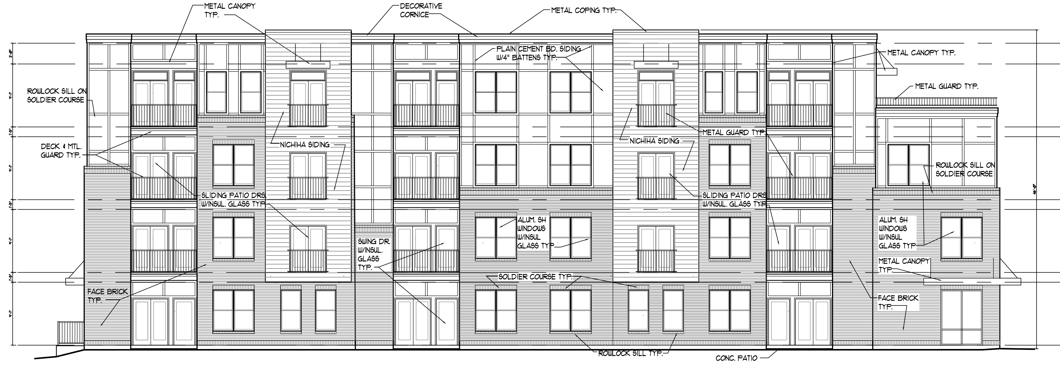
SOUTH FRONT ELEVATION SCALE: 1/8" = 1'-0"
